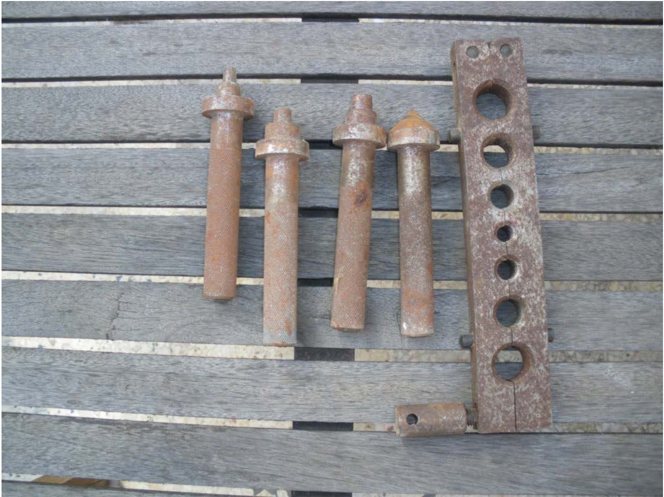
Beaten collar, tool used to flare copper pipes in plumbing, steel, dept 37 Renault in St Ouen, 1988, turned, drilled and milled. 3 hours of work.
