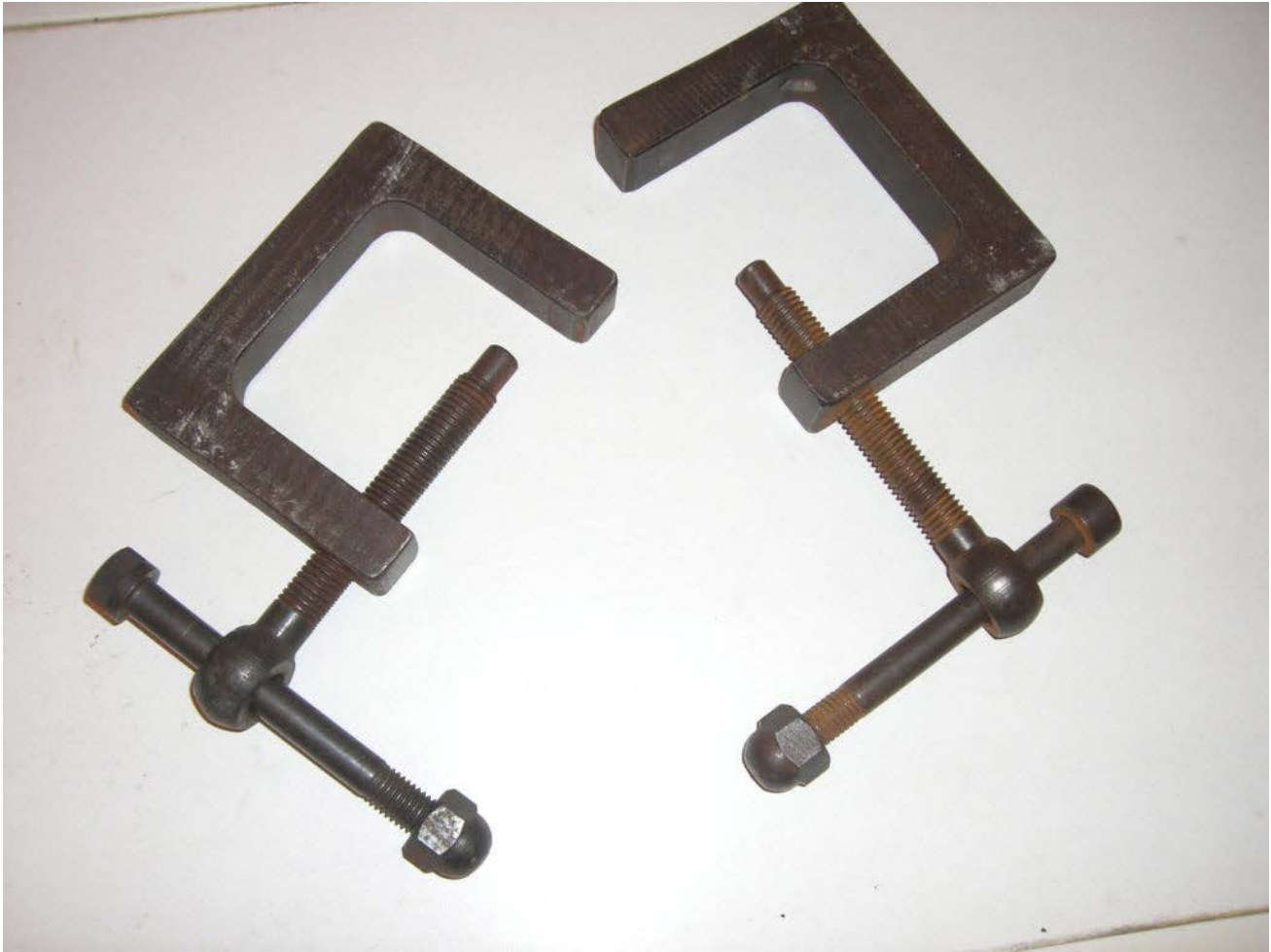
Clamps used to hold pieces, manufactured in the mid 80's at the wood dept 57 of the Renault Billancourt factories, steel, salvaged bolts and nuts assembled with two pieces of machined steel (about 3 hours of work), production: Marc Forestier, Robert Kosmann's photo collection.
