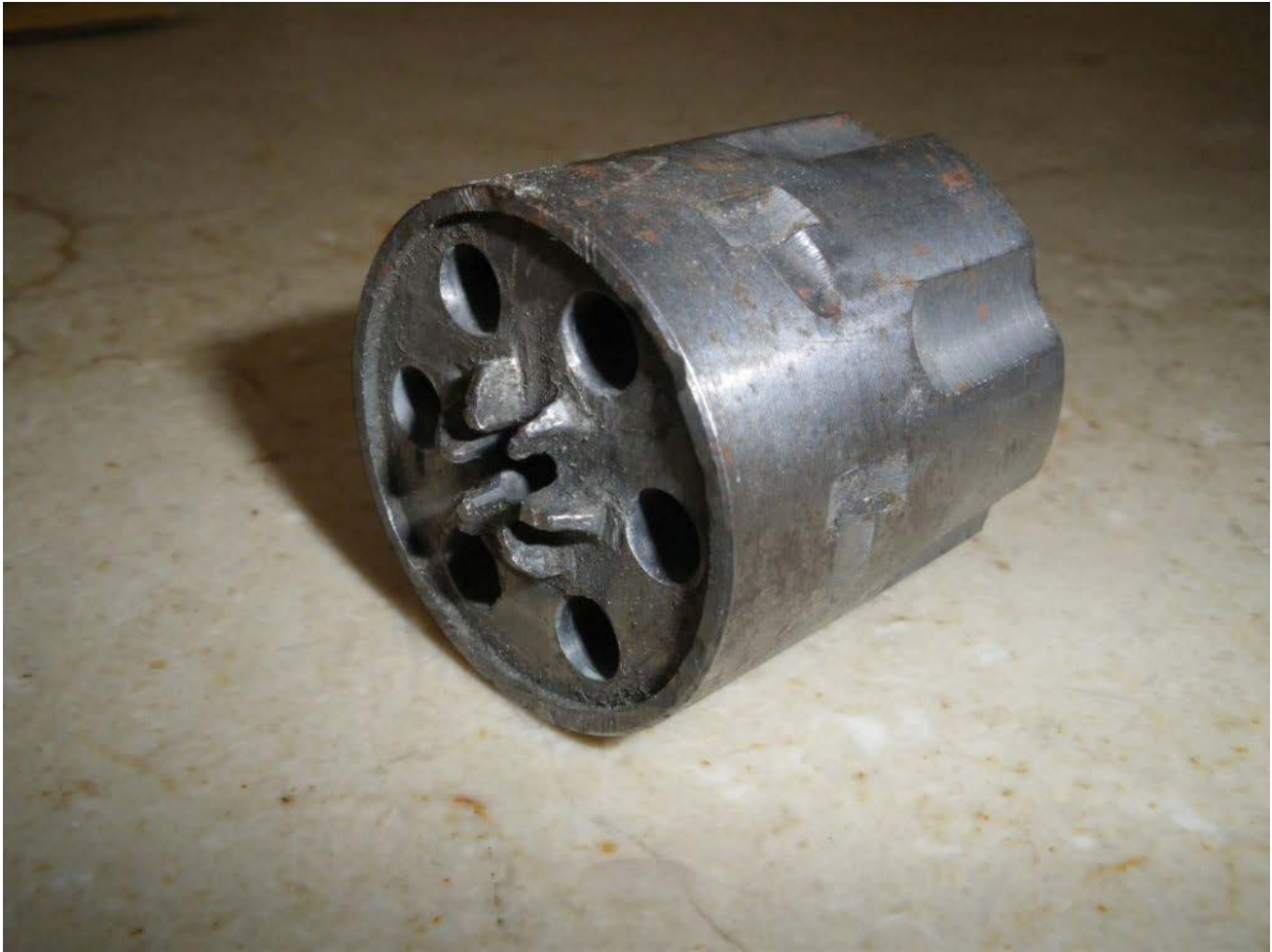
Cylinder manufactured in 1986 at St-Ouen's Renault plant, made of steel (turning + milling + fitting), about 5 hours of machining in total, serial production (4 copies) 2 for the homer-maker himself and 2 for those who helped him (welder, fitter). The cylinder is a copy of a single shot 22 long rifle that could be purchased freely at the time to turn it into a 6 shot 22 magnum. This was for private use, to shoot in the forest (weapons collector). Robert Kosmann's photo collection.
