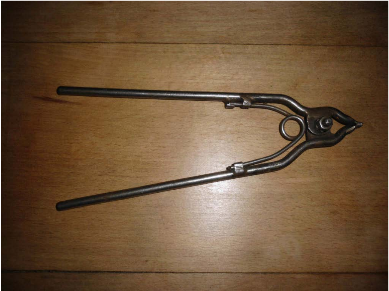
Circlip pliers, tool made at the Renault dept 70 in Billancourt, late 1970s, 22 cm, salvaged steel, shaping made by a fitter (about 5 hours of work), Patrick Schweizer's collection and photo.
